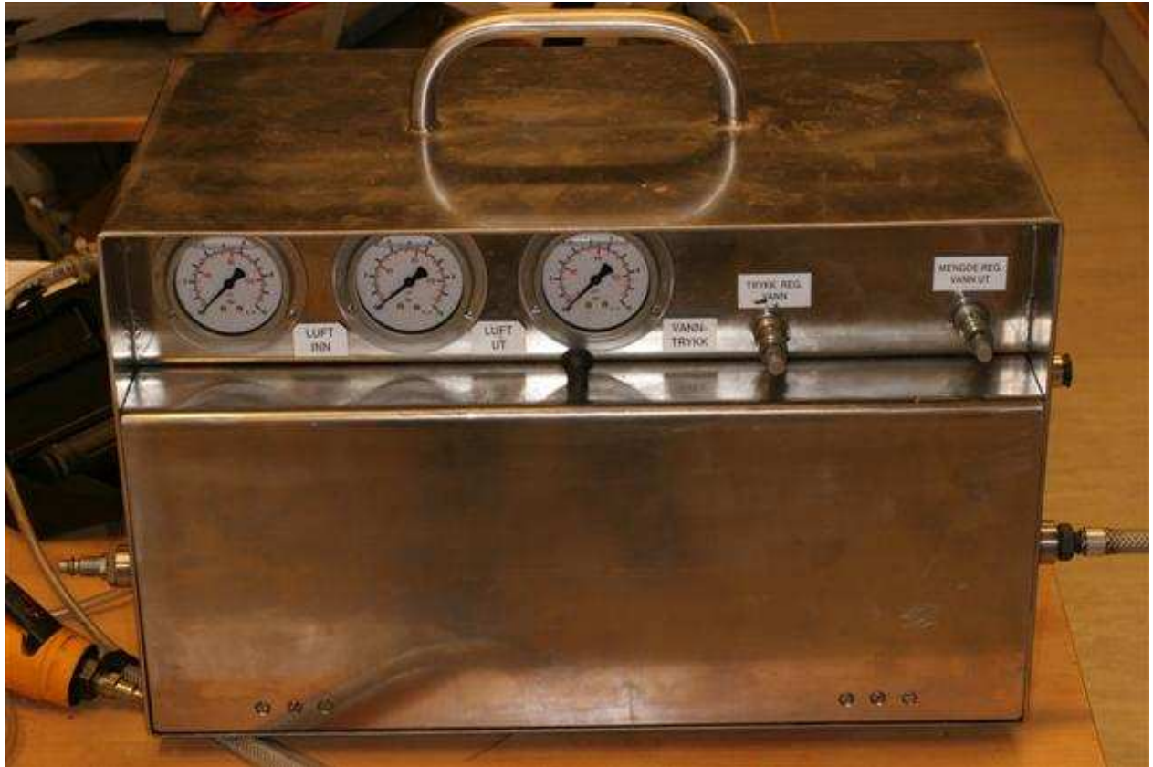
Water and pressurised air controller
