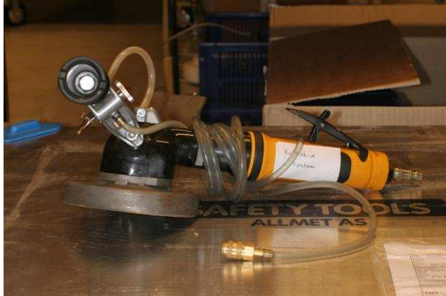
Cutting disc Atlas Copco air tool with water cooling
